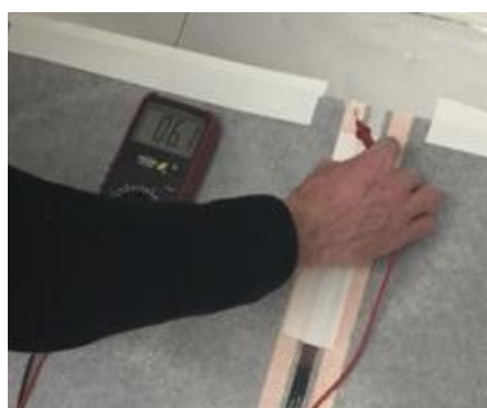
P19 Testing the heating film resistance
