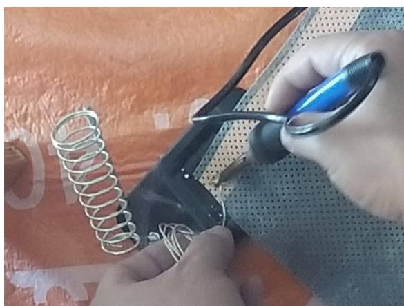
P8 Welding the wire to the heating film
